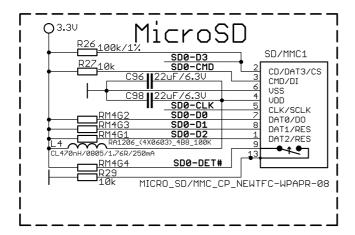
SD/MMC1 slot is the microSD card slot, located on the top of the board.
