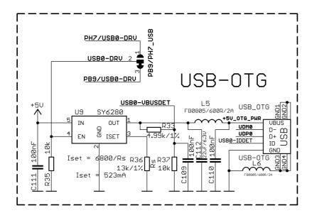
The USB\_OTG features Low Loss Power Distribution Switch SY6280 which protects the board in case the devices you have plugged to the USB\_OTG attempt to draw more current than 523mA
